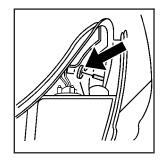
Carefully slide the taillamp assembly outward to clear the stud (see arrow) and then rearward and away from the body of the vehicle.
